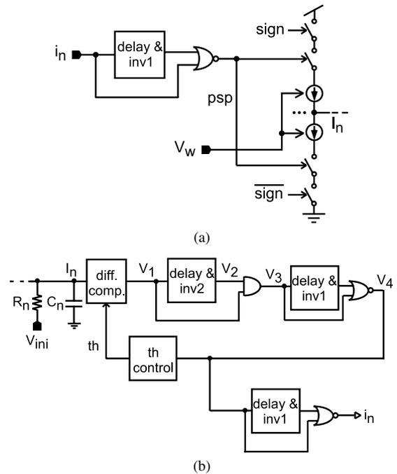
Fig. 4 Spiking neuron circuits: (a) synapse and (b) neuron.
